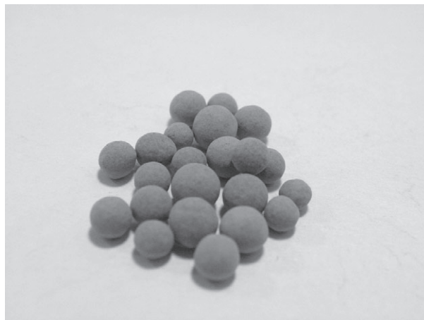
Fig. 2. C13 spherical methanation catalyst.
