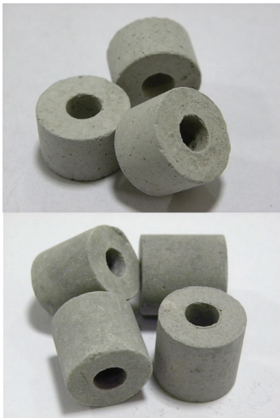
Fig. 9. C11-9-02 alpha-alumina reforming catalyst.
